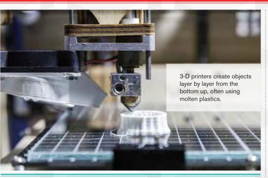
Home 3-D printers mostly use a process called, alternately, filament deposition manufacturing (FDM), fused filament fabrication (FFM), or fused filament fabrication (FFF), according to *Consumer Reports*, which conducted lab tests on three different models of home printers. With this method, plastic filament (basically a thin cord that comes in rolls) is pushed through a heated "print head" that produces ("extrudes") molten plastic or nylon in thin layers to produce an object.
