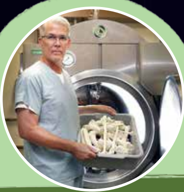
Dean Fisher, Director of the Donated Body Program at UCLA, shows off the Resomator machine, which strips the bones clean. The bones are then pulverized and can be placed into an urn, just like in flame cremation. Photos courtesy of MOVI Inc.
